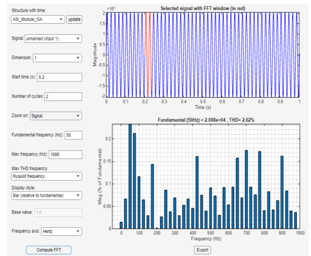
Figure 6e: THD of Grid Current
