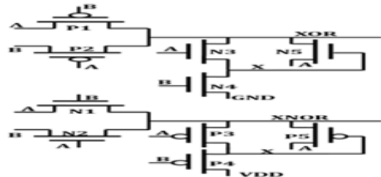
Fig.4. Proposed XOR-XNOR circuit for Full Subtractor
