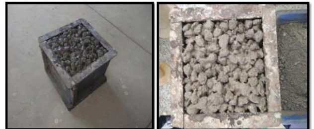
Fig .2. Casting of cube specimen
