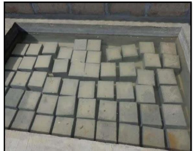
Fig.3. Curing of cubes
