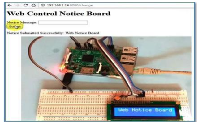
Fig.5. Web Controlled Notice Board Setup
