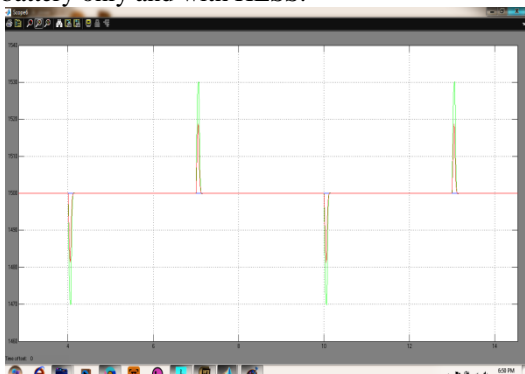
Fig 7: The propulsion motor speed without ESS, with battery-only and with HESS.
