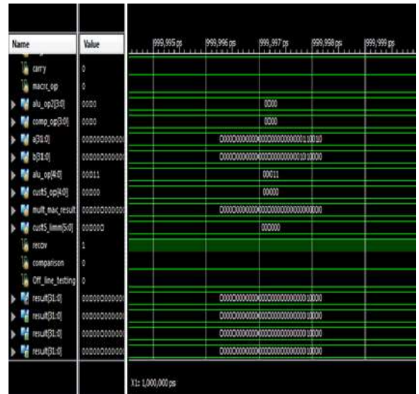
Fig 8: Simulation result of recovered modefor AND operation of two variables using SMERTMR.
