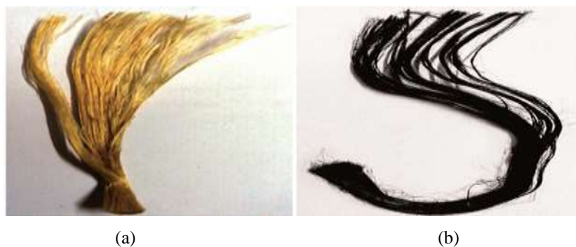
Figure 1: Digital images (a) unmodified and (b) modified Adavibenda fibers with in situ generated AgNPs by hydrothermal method
