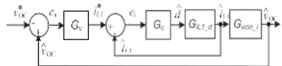
Fig. 4. Double loop current-mode control structure
