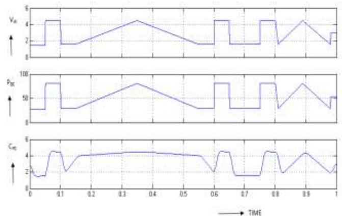
Fig.7. Performance of WECS with proposed MPPT algorithm for Dynamic response under varying wind conditions.
