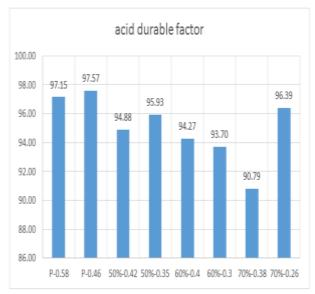
Acid durable factor is more for plain concrete. In fly ash concrete acid durable factor high for 50% replacement. The acid durable actor for M30 grade of concrete for 50%, 60%, 70% replacement of fly ash 11.44, 22.49%, 46%, low, when compared with plain concrete at the curing period of 28 days. The acid durable factor for M40 grade of concrete for 50%, 60%, 70% replacement of fly ash 5.81%, 15.73%, 19%, low, when compared with plain concrete at the curing period of 28 days.
