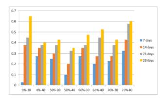
Diagonal loss is more for specimens with 70% replacement of fly ash. Compare with the plain concrete and among all the percentage replacement, 50% replacement of fly ash shows less mass loss.
