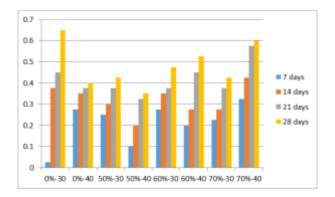
With the addition of fly ash resistance against the acid attack has improved. Acid attack factor is low for specimens with replacement of 50%, but for 7 days plain concrete (M30 grade) shows low acid attack factor.
