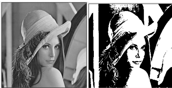
(b) DDBTC coding with minimum and maximum values and with 0s and 1s
