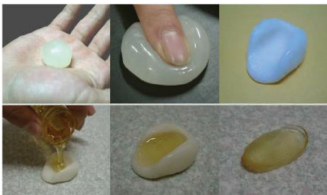
Figure 1 : Making an artificial fingerprint directly from a live finger plastic is used to obtain the mold and gelatin to obtain the cast.
