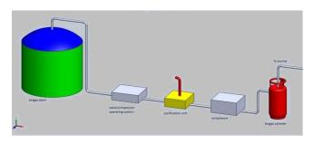
The gas from the chamber is first subjected to pressure test and when pressure range is in the desirable region the valve open and also the compressor started .The gas is being sucked and pass through the purification unit (hollow fiber membrane) ,the  $co_2$  get separated and compressed to a storage tank . The purification unit remove the unwanted gases, it reduce the quantity which is to be compressed to the storage tank by the compressor
