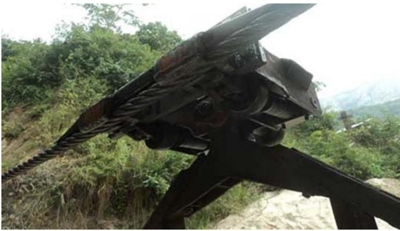
Fig. 2 The carriage & detachable grip of the ropeway system
