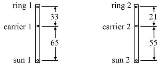
Figure 2(b):Lever representation of each gear set
