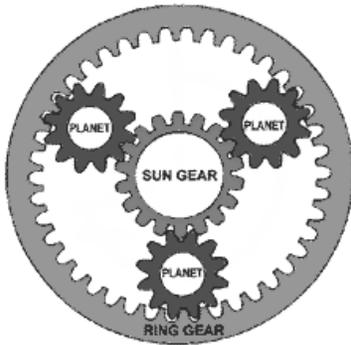
Figure 1: Planetary Gear System
