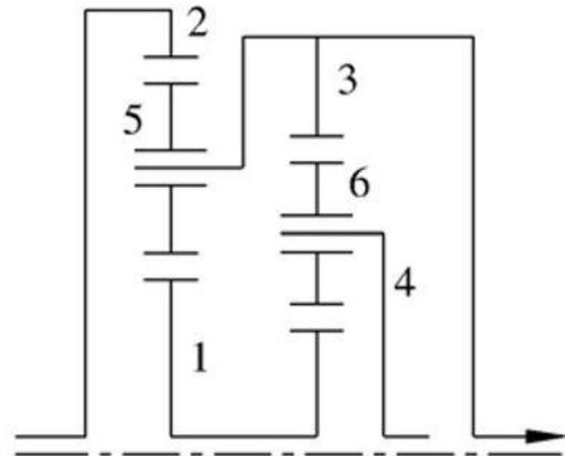
Figure 4: Alternative configuration for Simpson Gear train
