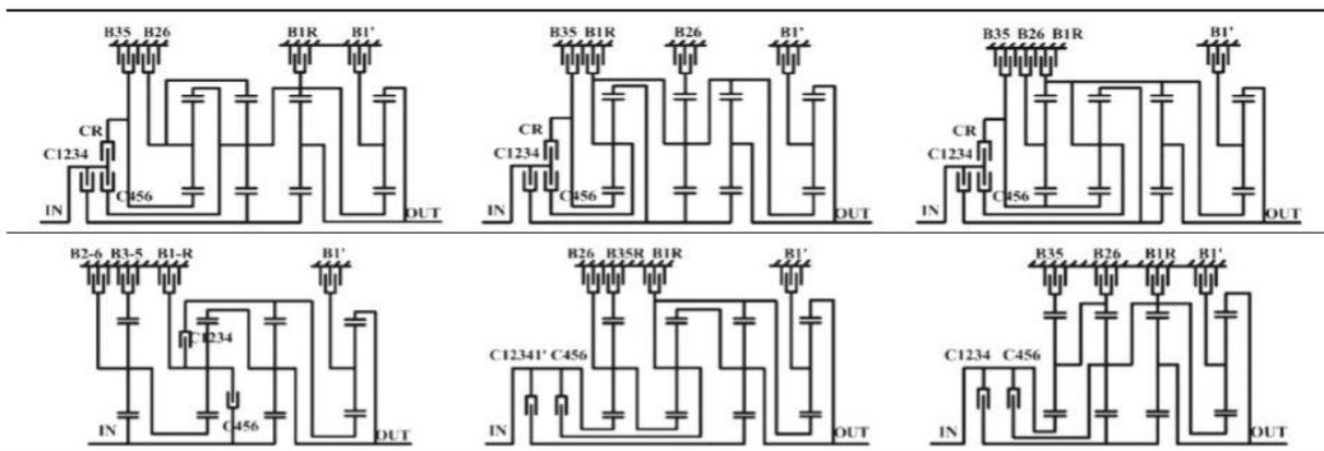
Figure 10: Stick diagram of seven speed PGTs.
