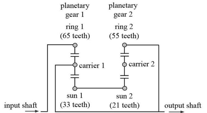
Figure 2(a): A stick diagram of two connected planetary gear sets
