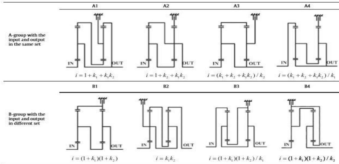
Figure 9: Stick diagram of 2-PGs PGTs with high reduction speed ratio.
