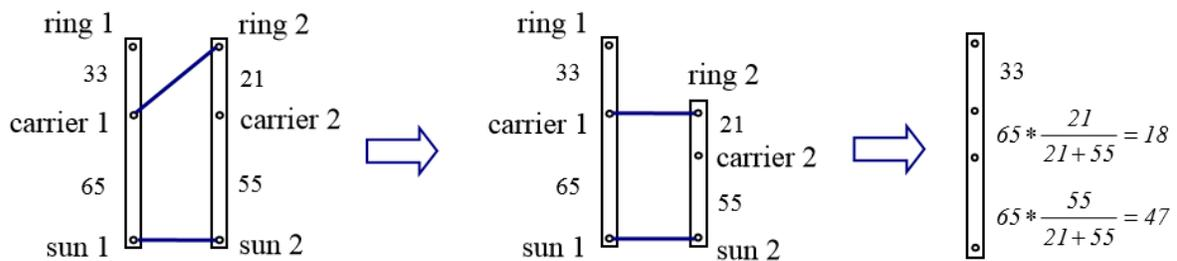
Figure 2(c): Two connected gear sets and lever representations
