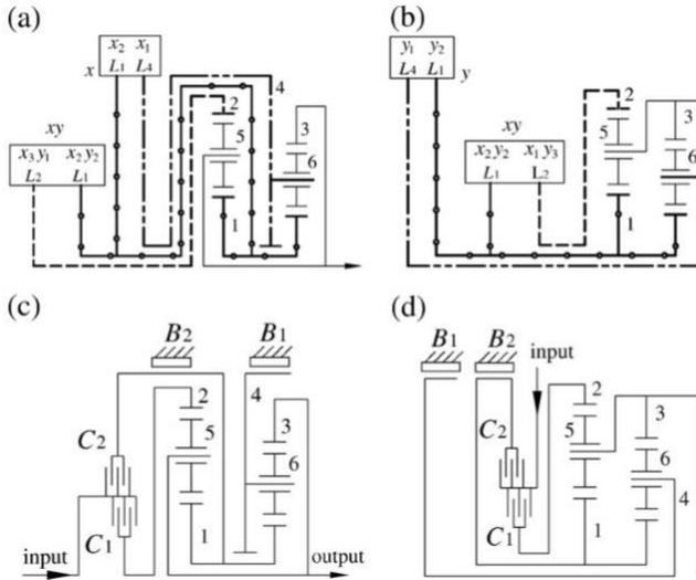
Figure 5: Coded layouts and stick diagram
