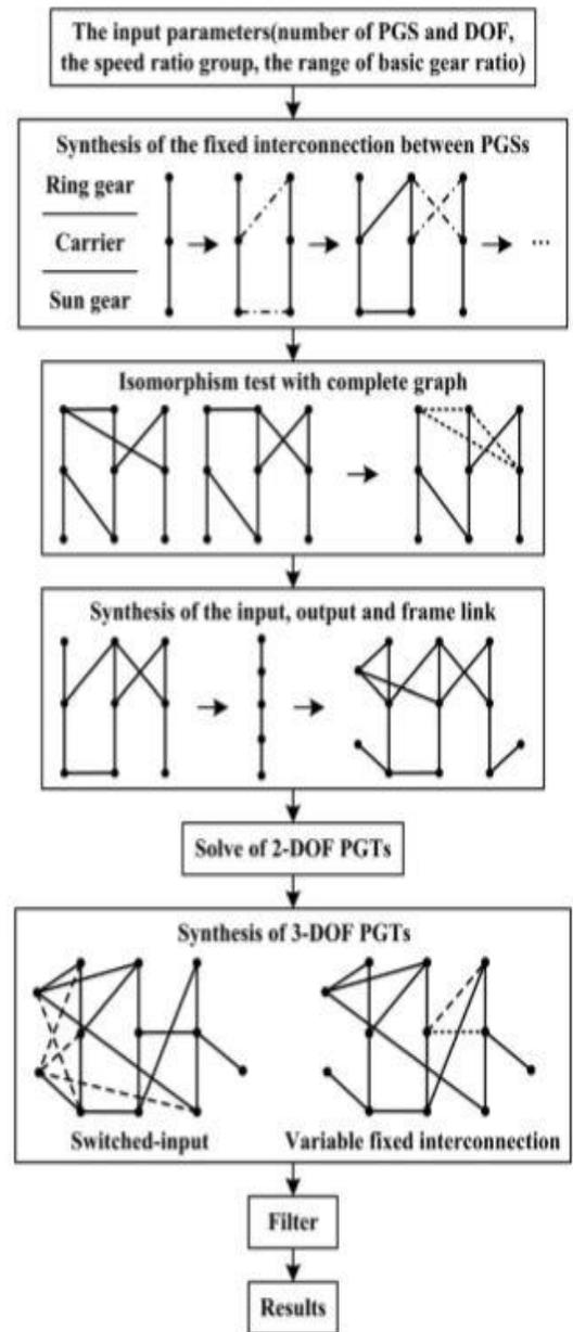
Figure 8: Synthesis Algorithm for seven speed PGTs
