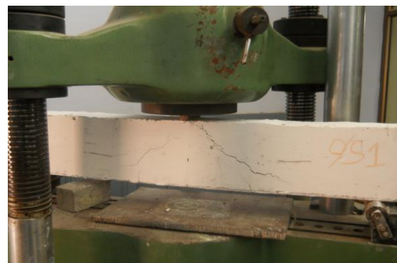
Fig: 5.2 Flexure Failure of under reinforced concrete beam
