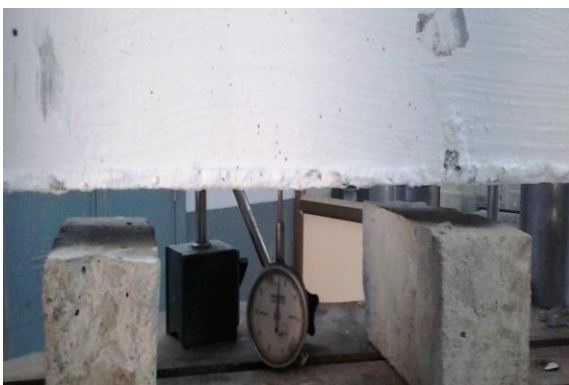
Fig.3.3 Dial gauge arrangement for testing beam
