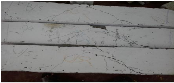
Fig: 5.4 Flexure Failure of over/balanced/under reinforced concrete beam
