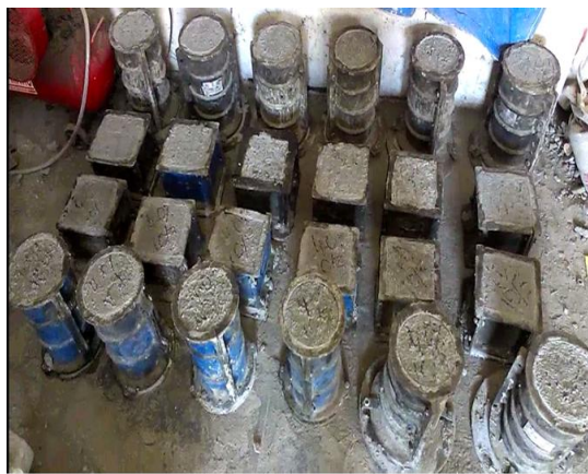
A VIEW OF CAST SPECIMENS IN MOULDS
