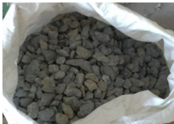
A VIEW OF THE DEMOLISHED AGGREGATE USED
