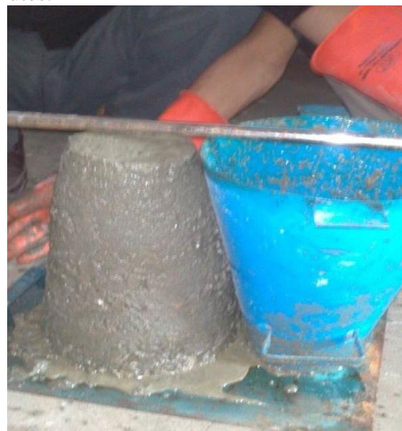
VIEW OF SLUMP CONE TEST
