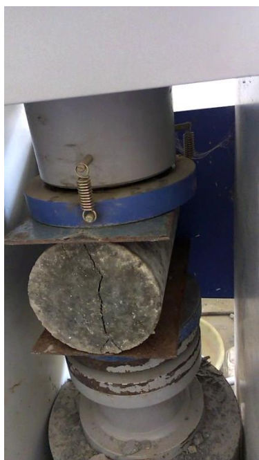
VIEW OF SPLIT TENSILE STRENGTH TEST OF CYLINDER
