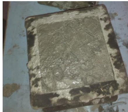
FRESH CONCRETE IN THE MOULD
