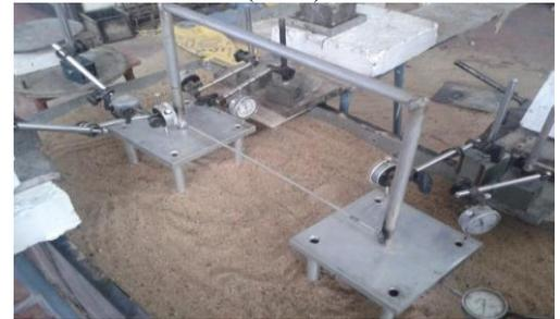
Figure 3.16: Photograph of Model plane frame at base (5mm)
