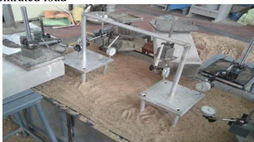
Figure 3.6: Photograph of Model plane frame at arrangement of dial gauge
