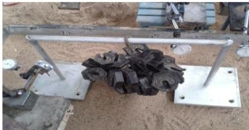
Figure 3.4: Photograph of Model plane frame at central concentrated load
