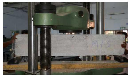
Figure 3.2.1. The Three point bending beam specimen for mode -I fracture
