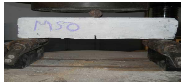
M 50 -Small beam before loading
