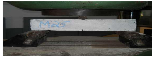
M25-Small beam before loading
