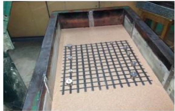
Figure 3.3: Placing of geogrid
