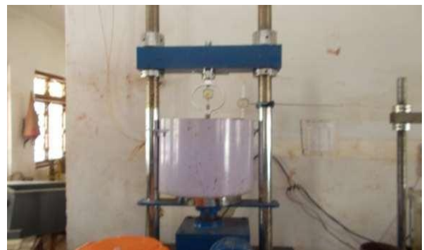
Fig .2. The Footing Load Test Machine
