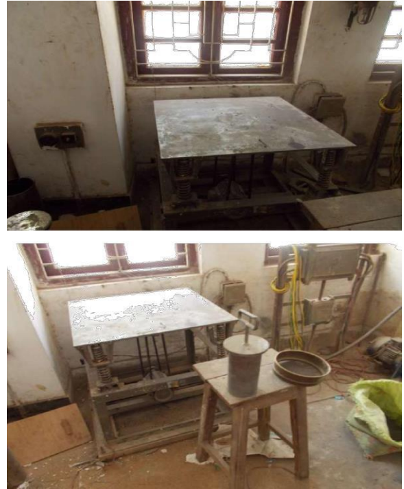
Fig 1. The Vibrating Table Along With The Hammer
