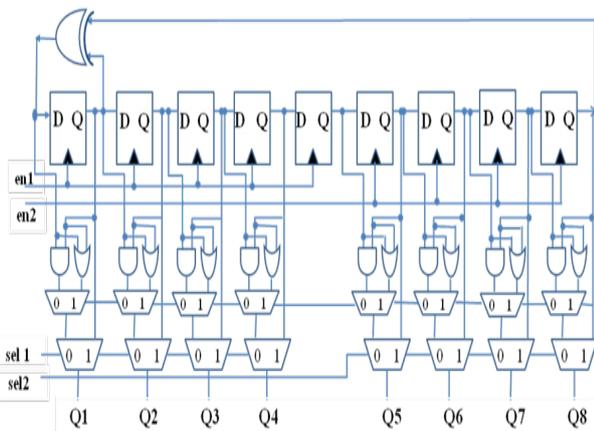
Fig 3. Internal structure of 8-bit LP-LFSR
