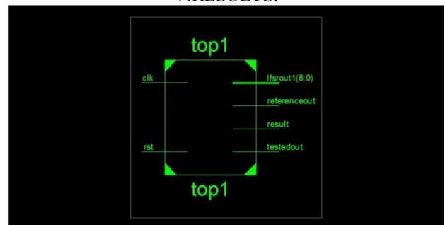
Internal RTL Schematic
