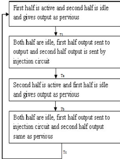
Fig 4. Proposed algorithm for low power LFSR
