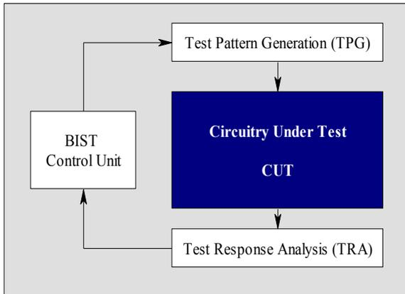
Fig 1 Test Pattern Generator
