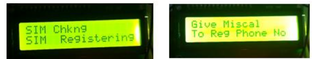
Fig.4. A number has to be registered by giving miss call to the number placed in the GSM Modem in order to communicate to if incase an accident occurs.
