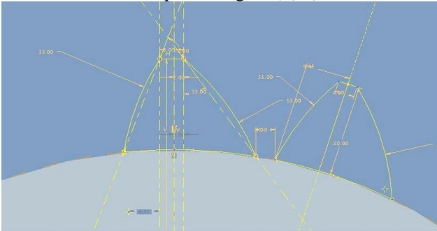
ASYMMETRIC GEAR (pressure angle 350) (2D)
