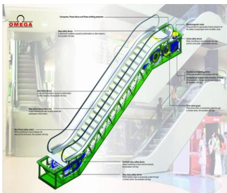
Fig 1. Model of the Escalator and its frame
